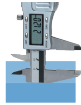
Stufenmessung/ step measuring
