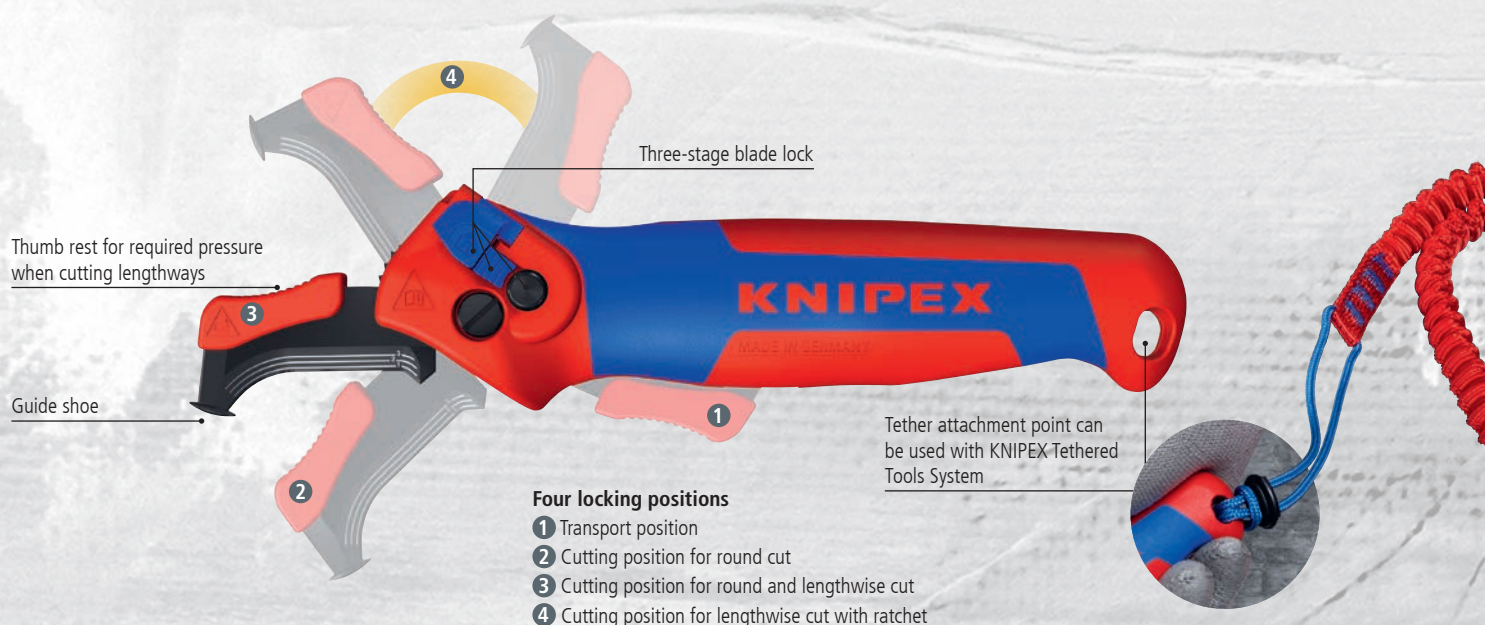
Ratchet function enables stripping with more comfort and less effort
