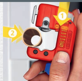
... preset with the scale and click onto the tube with the spring-loaded cutting wheel
