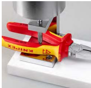
Pressure test at 70°C.
