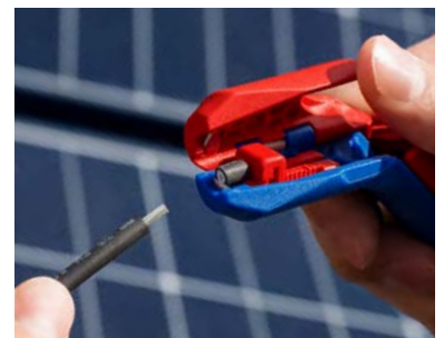
16 95 03 SB: Length stop for PV cables: Adjustable from 6- 18 mm for reproducible stripping lengths, suitable for all common PV connectors
