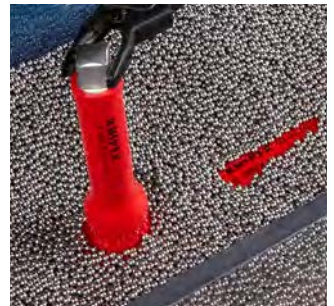
Testing the electrical insulating properties.
