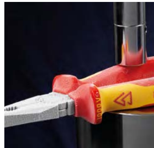
Cold impact test at -25°C.
