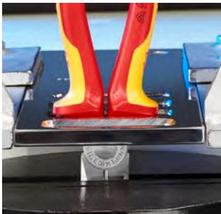
Testing the adhesion of VDE sleeves with 500 N at 70°C.
